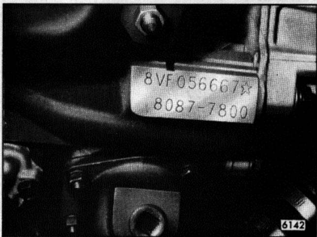
Fig. 4. Typical 6V-92 and 8V-92 Engine Serial Number and Model Number as Stamped on Upper Right Front Corner of Cylinder Block
