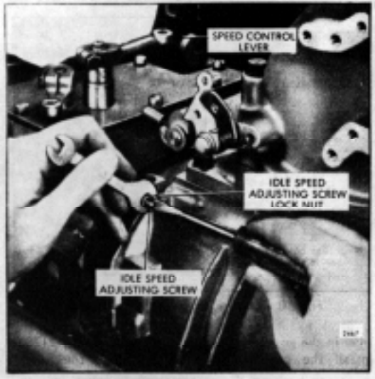
Fig. 7. - Adjusting Engine Idle Speed
